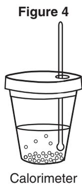
A thermometer is inserted through the lid. The copper and water are gently stirred in the cup. The temperature is checked periodically. The highest temperature noted is 26.3°C.
